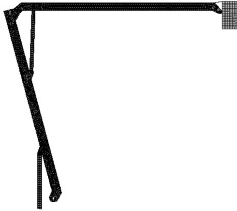
Fig. 3. Finite element model of aloft working vehicle
